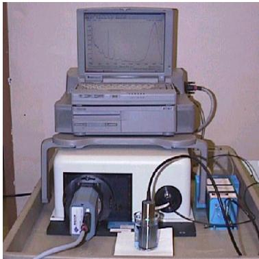
Charged-coupled devices (CCDs) used as detectors for Raman spectroscopy have little quantum efficiency at wavelengths above 1000 nm. It was important for this project that an appropriate excitation laser wavelength was selected to provide ample spectral range while avoiding
